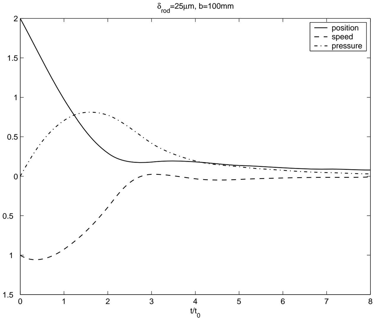
Figure 3.3: Results of simulation with small leakage: the gap width  $\delta_{\text{rod}} = 25\mu\text{m}$ . Position, speed and pressure refer to the non-dimensionalised variables,  $x_1$ ,  $x_2$  and  $x_3$ , respectively. These related to the dimensional quantities via (3.4).
