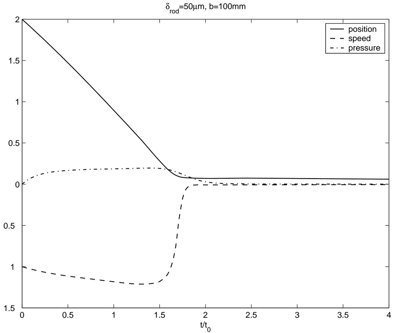
Figure 3.2: Results of simulation with moderate leakage: the gap width  $\delta_{\text{rod}} = 50\mu\text{m}$ . Position, speed and pressure refer to the non-dimensionalised variables,  $x_1$ ,  $x_2$  and  $x_3$ , respectively. These related to the dimensional quantities via (3.4).
