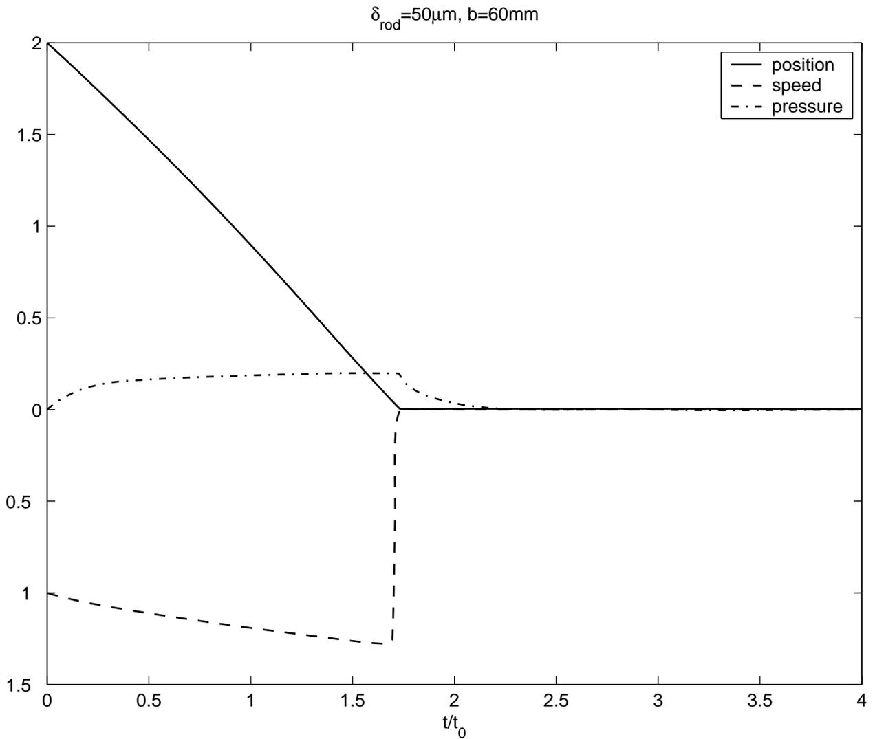
Figure 3.5: Results of simulation with moderate leakage: the gap width  $\delta_{\text{rod}} = 50\mu\text{m}$ , and the flange width  $b = 60\text{mm}$ . Position, speed and pressure refer to the non-dimensional variables,  $x_1$ ,  $x_2$  and  $x_3$ , respectively. These related to the dimensional quantities via (3.4).
