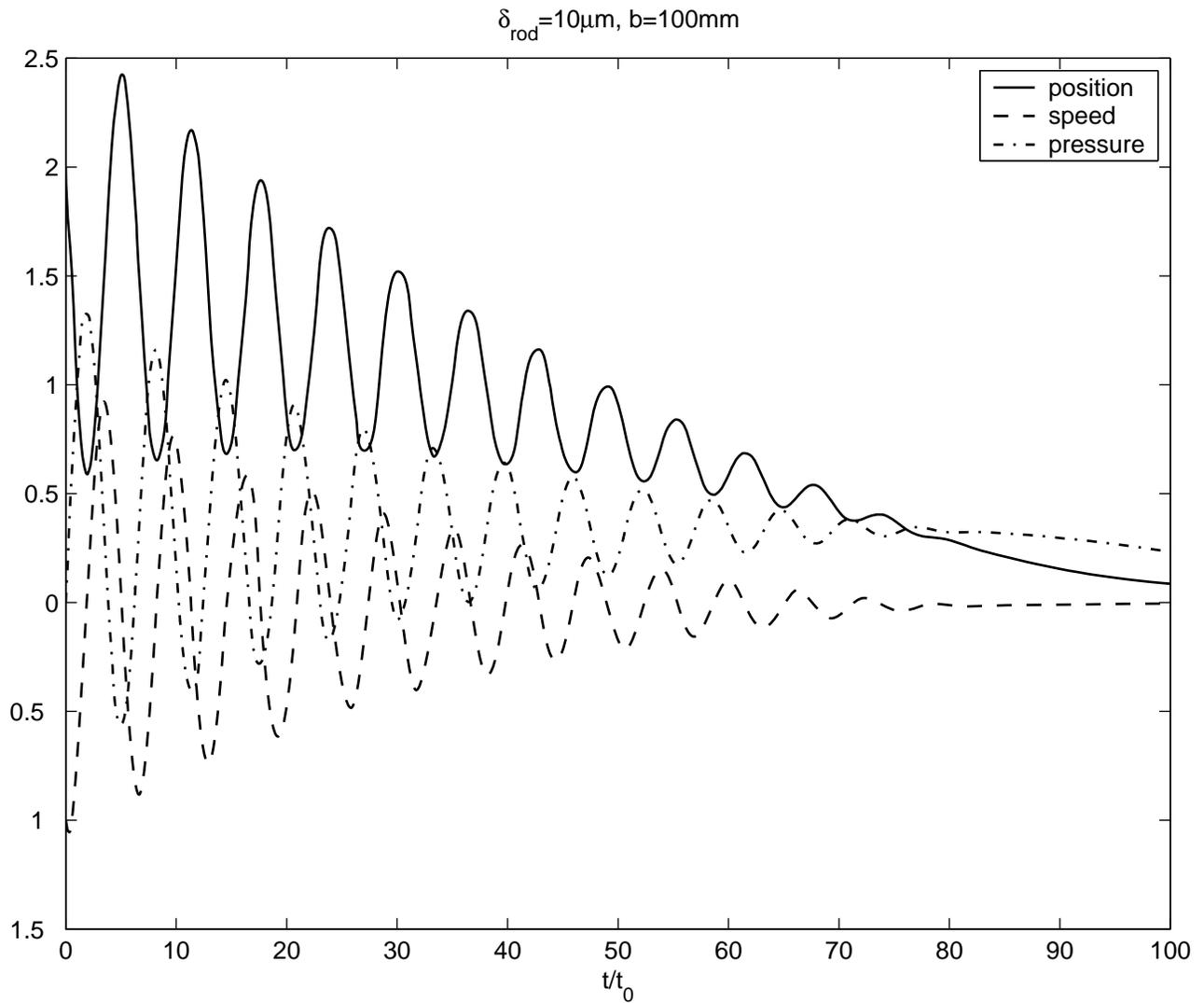
Figure 3.4: Results of simulation with extremely small leakage: the gap width  $\delta_{\text{rod}} = 10\mu\text{m}$ . Position, speed and pressure refer to the non-dimensionalised variables,  $x_1$ ,  $x_2$  and  $x_3$ , respectively. These related to the dimensional quantities via (3.4).
