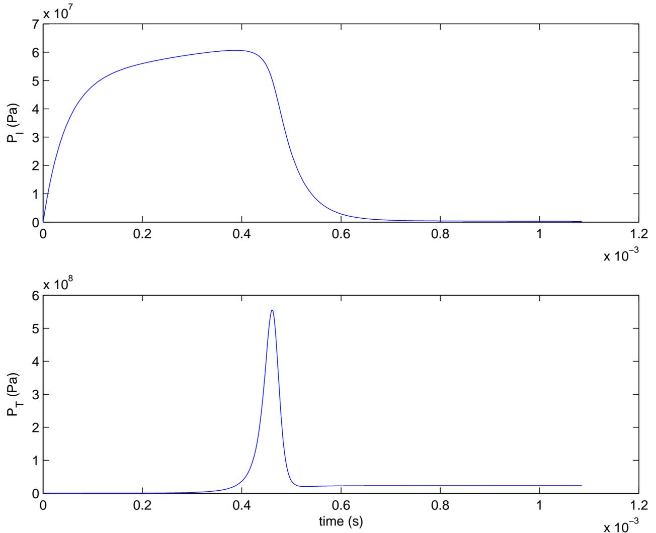
Figure 3.6: Pressure in mold  $P_I$  and pressure (spatial maximum) in squeeze film  $P_T$  vs. time for the parameter values the gap width  $\delta_{\text{rod}} = 50\mu\text{m}$ , and  $b = 100\text{mm}$ .
