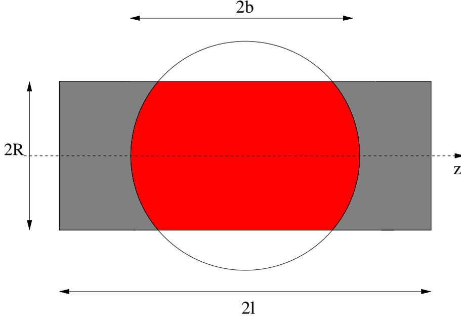
Figure 3: A plan view of the surface given by the laser light intersecting the cylinder
