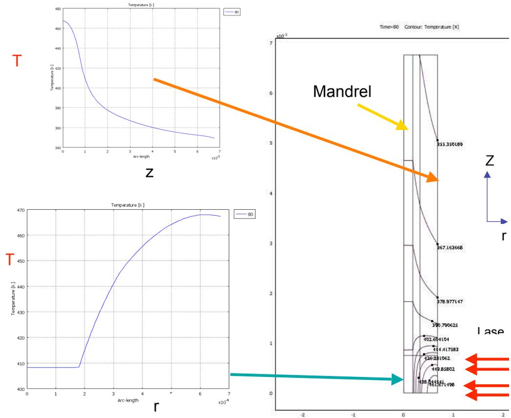
Figure 2: A numerical approximation to the solution obtained by using the Finite Element method at the time  $t = 80s$ . In this calculation the contours of the temperature are given on the rightmost figure in which the radial direction is horizontal and the axial direction is vertical. The system is heated by the Laser at the bottom right corner. The other two figures show the axial surface temperature (top) and the radial temperature through a cross-section (bottom)
