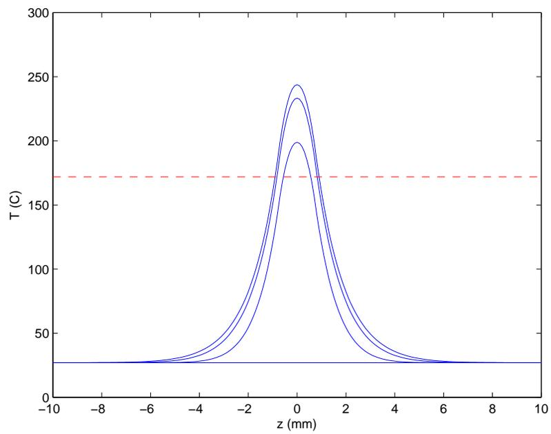
Figure 5: The averaged temperature  $\bar{T}(z, t)$  as a function of  $z$  for various times  $t = 0s, 10s, 20s, 30s$ . The melting point of the Pebax is indicated by the dotted line
