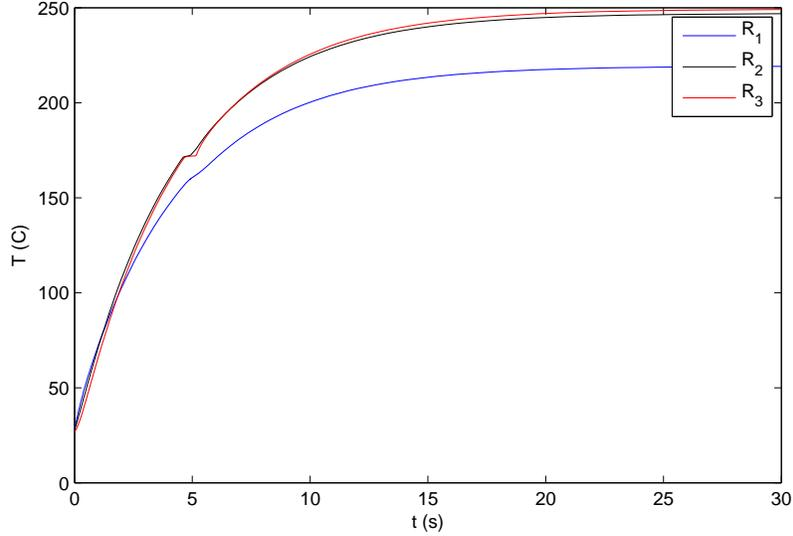
Figure 4: The change in temperature with time at radii  $R_1 < R_2 < R_3$ . Note the effect of the phase change leading to the welding and the associated polymer bond.
