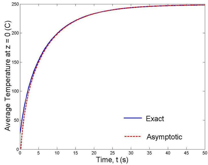
Figure 6: The centre temperature  $\bar{T}(0, t)$ , comparing the exact and the asymptotic solutions.
