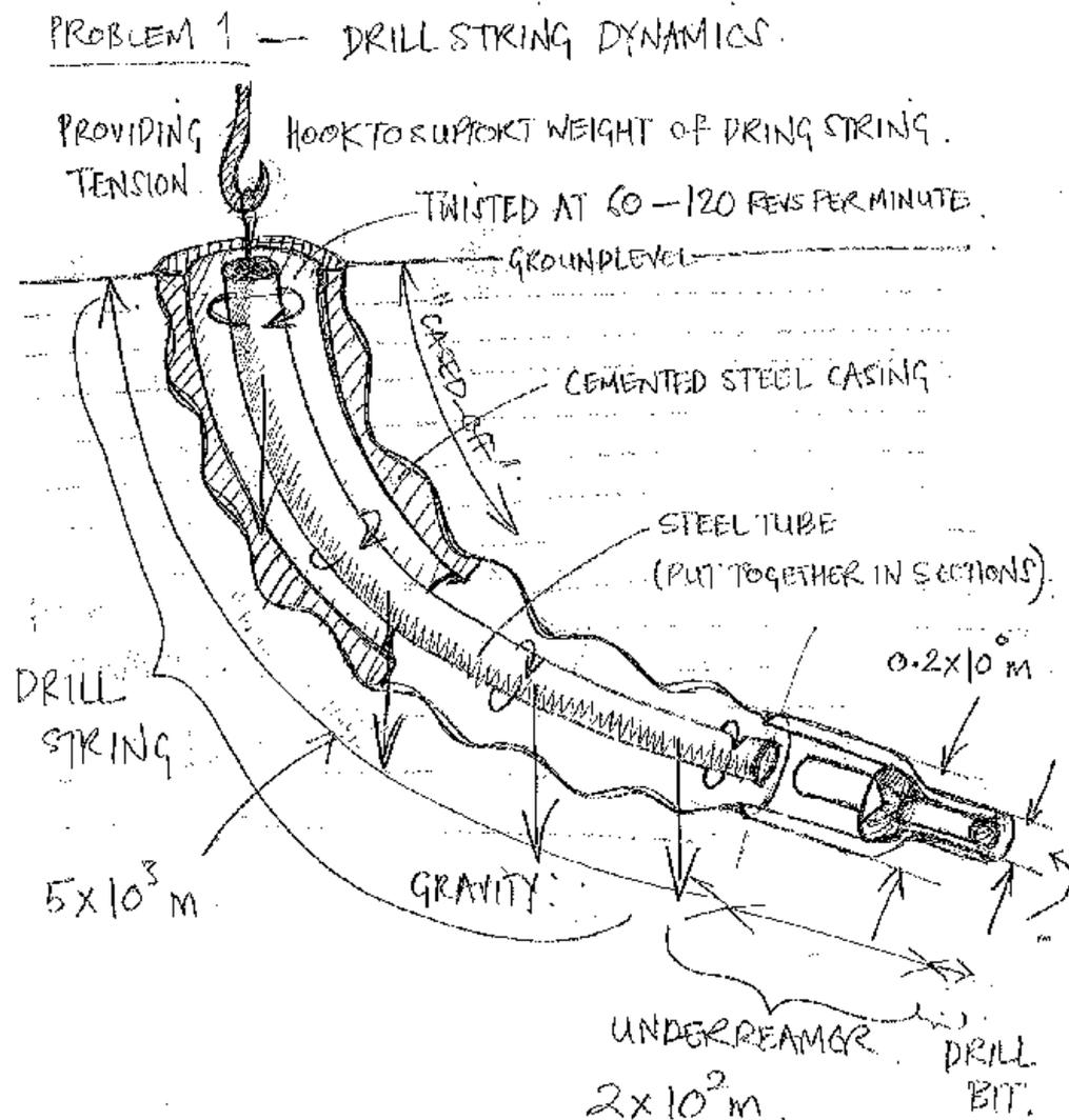
**Figure 2:** Schematic of drillstring dynamics problem
