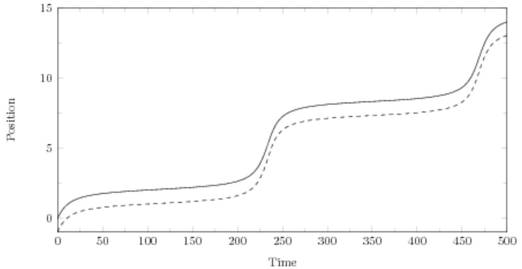
**Figure 7:** Progress of drill-bit (shown as continuous line) and underreamer (shown as dashed line), when  $R(x) = 0.9 + 0.12 \sin x$  and all other constants are taken to be one. Note that the drill-bit and underreamer become effectively stuck for large periods of time, before breaking through the formation and continuing.
