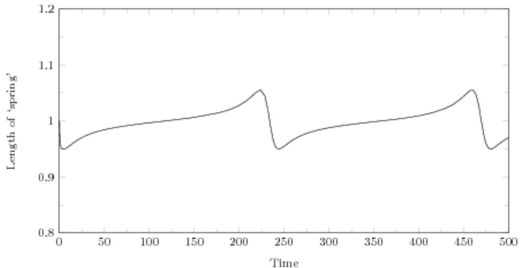
**Figure 8:** A plot of  $g(t)$  over time, showing the changing length of the material connecting the drill-bit and the underreamer. This effectively acts as a spring, moderating the forces between the drill-bit and the underreamer.
