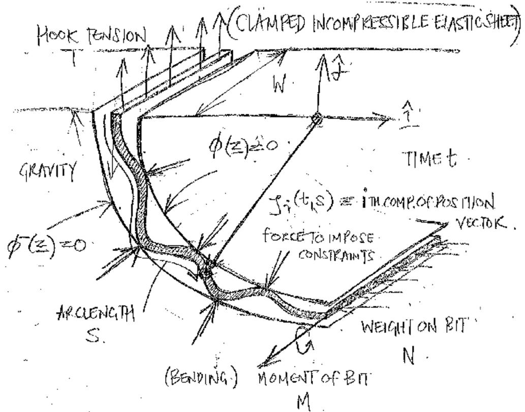
Figure 3: Schematic of planar model
