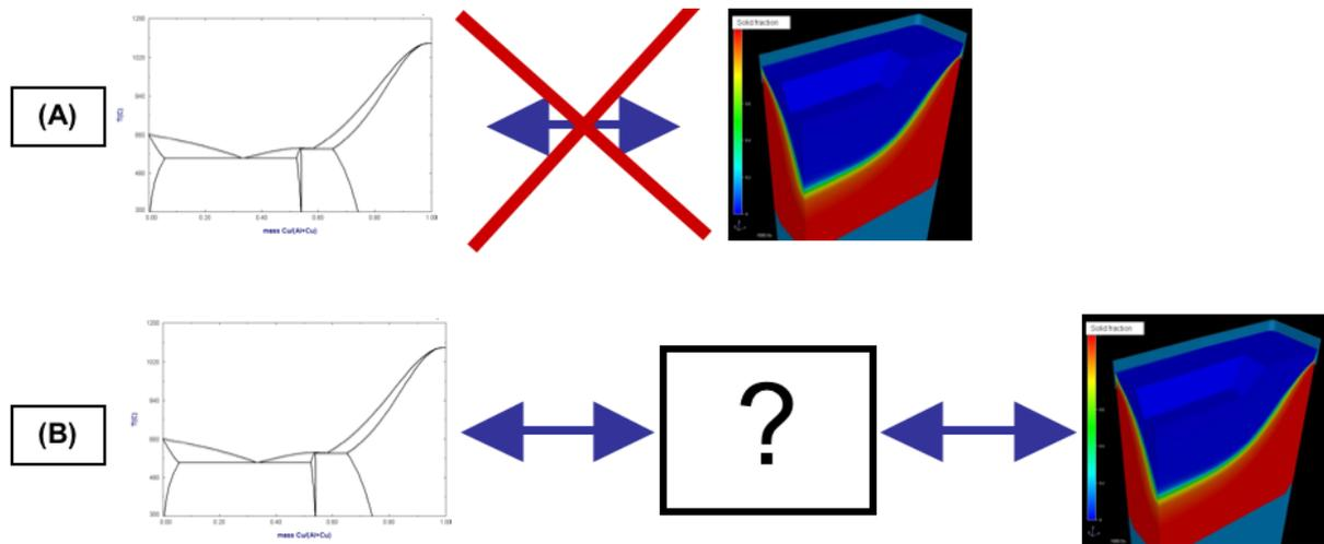
Figure 3: The Corus challenge: Composition needs to be included in casting modelling. (A) Direct coupling between thermodynamic software and the simulation is too time consuming. (B) The challenge is to propose efficient coupling step(s) between the simulations and the thermodynamic database.
