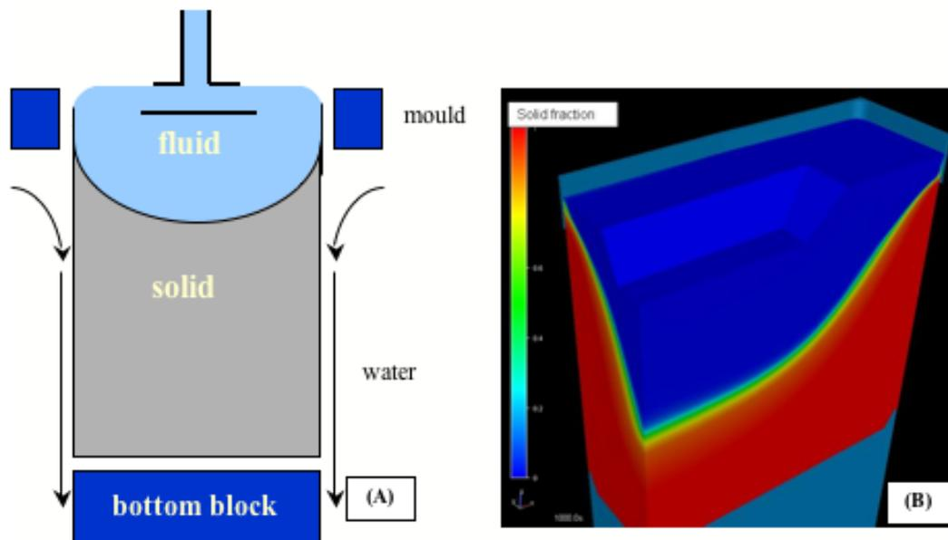
Figure 1: Schematic of the semi-continuous aluminium casting process (A) and Alsim model prediction (B) showing one quarter of an ingot during casting. The colour change shows the transition from liquid (blue) to solid (red) in the casting process.
