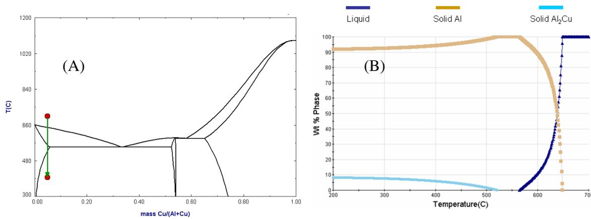
Figure 2: Solidification and phase formation during cooling of an Al-Cu mixture. The phase diagram (A) gives the relation between phases, composition and temperature. (B) shows the phase formation during solidification of Al with 4.5 wt% Cu, also indicated by the green line in (A).
