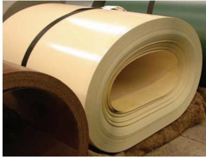
(a) Colorbond steel coil with race-track bottom
