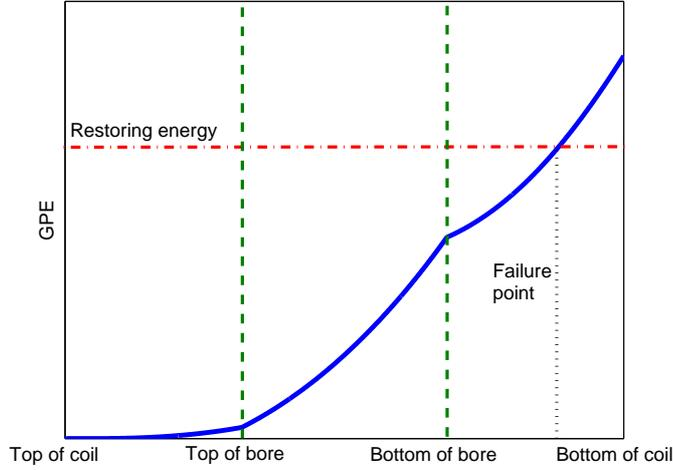
Figure 5: Gravitational potential energy of the self-weight of a coil
