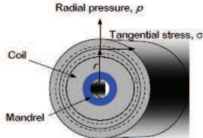
Figure 1: Basic Coil Geometry
