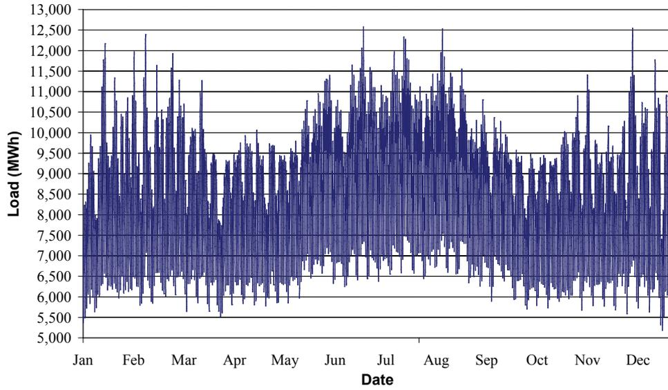
Figure 3: NSW State Half-hourly Electricity Demand in 2005 (MWh)
