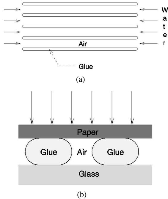
Figure 9: Processes in competition when removing of the labels.
