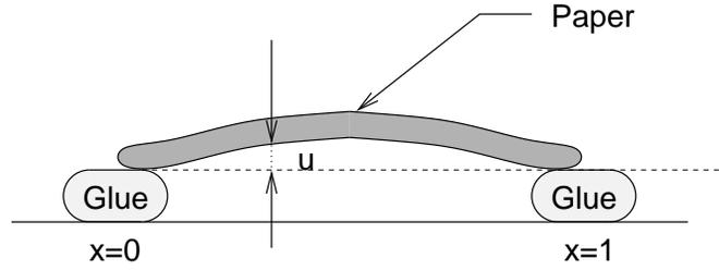
Figure 4: Typical configuration for the Euler strut.
