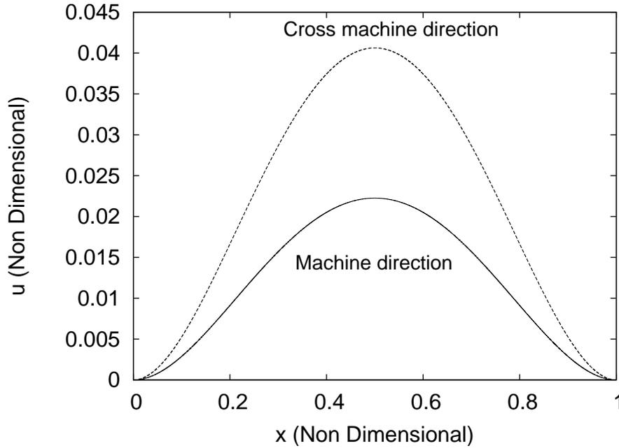
Figure 8: Paper expansion in machine and cross machine directions.
