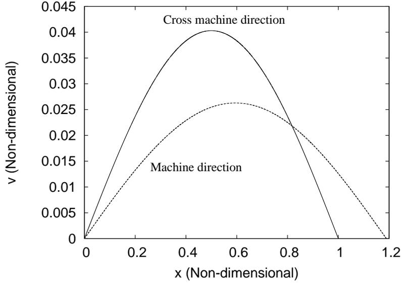
Figure 5: Paper expansion in machine and cross machine directions.
