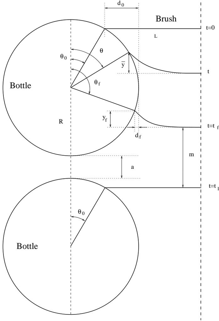
Figure 1: Geometry of brush on beer bottle.
