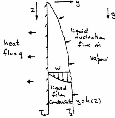
Figure 3. Flow of a laminar condensate film over a vertical plate
