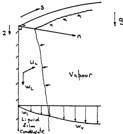
Figure 4. Flow over a curved vertical plate
