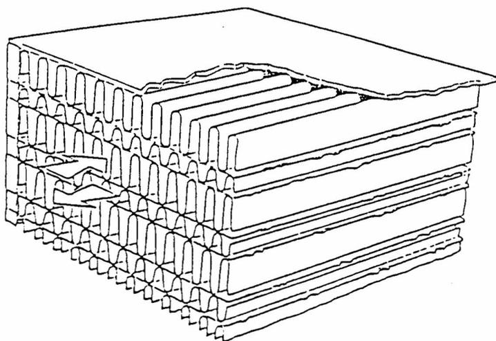
Figure 1. Plate-fin heat exchanger cross-section
