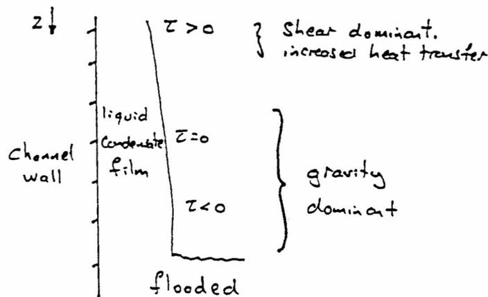
Figure 5. Schematic development of a film on a channel cross-section
