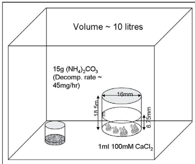
**Figure 2** Experimental apparatus for the gas diffusion process.
