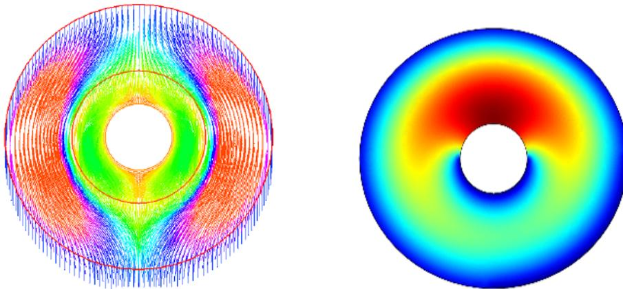
**Figure 3:** Flow field (left) and species concentration (right) in a porous medium with a blockage. Red colours denote higher values, the flow is from top to bottom.
