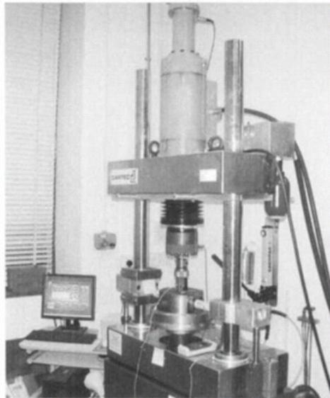
**Figure 5:** Experimental apparatus for determining contact coefficients
