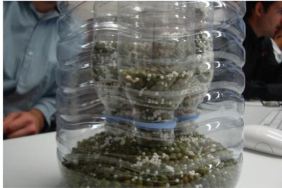
**Figure 3:** Experimental Setup #3: Three inlets pouring from a variable height above the piles.
