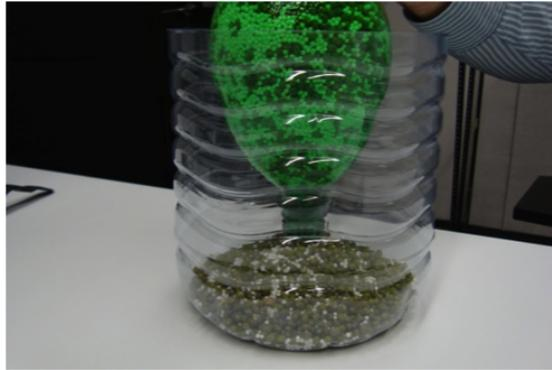
**Figure 4:** Experimental Setup #4: One inlet pouring from a variable height above the pile.
