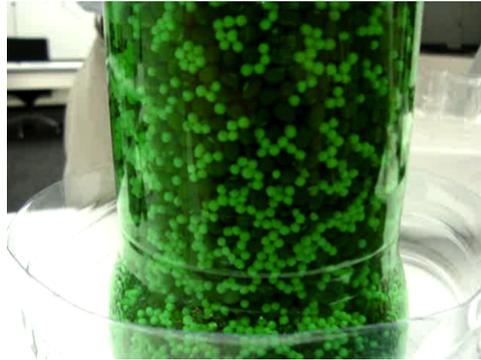
**Figure 2:** Experimental Setup #1: Draining a cylinder with a conical outlet.
