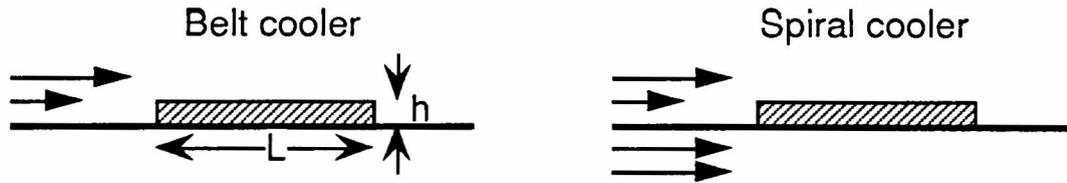
Figure 1: The geometries of typical industrial coolers
