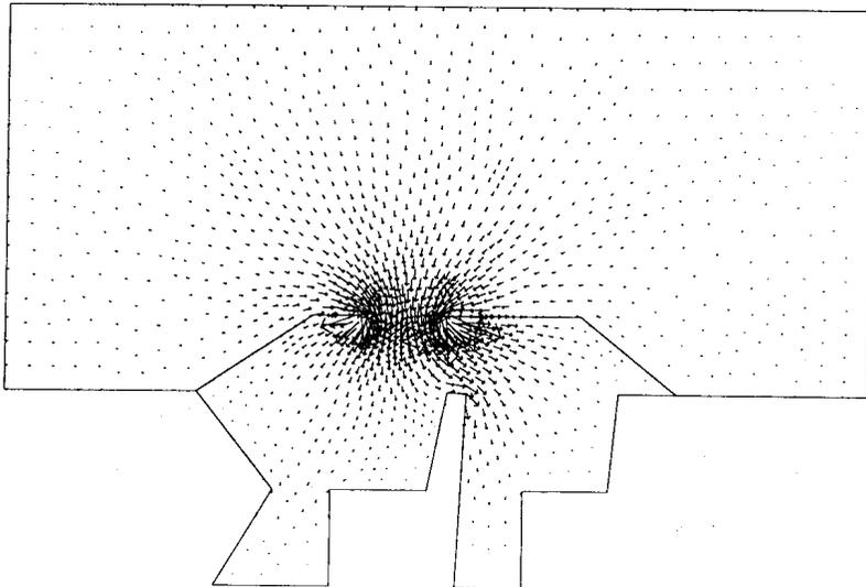
Figure 5: Velocity vectors for acoustic mode
