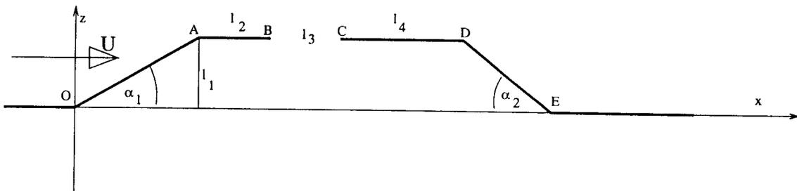
Figure 3: Representative geometry of windscreens and roof
