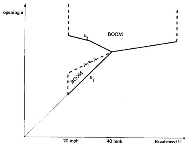
Figure 1: Typical behaviour of  $a_1$  and  $a_2$ , the openings for first and second onset of boom as functions of road speed  $U$ .
