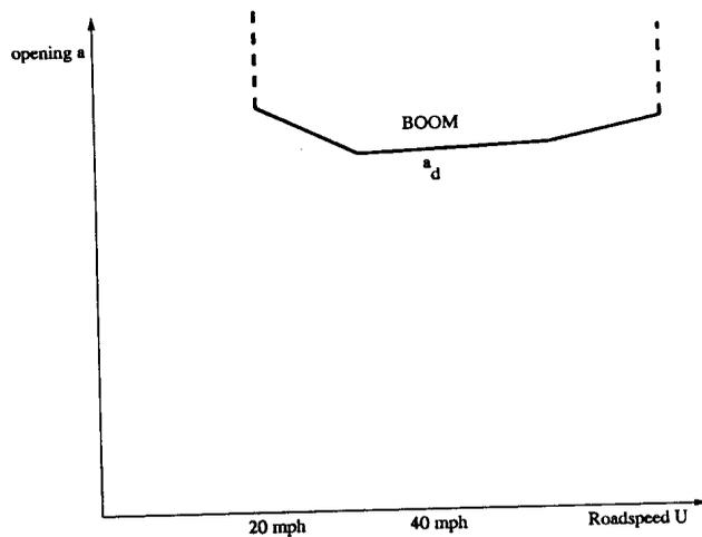
Figure 2: Typical behaviour of  $a_d$ , the opening at which boom occurs when a deflector is used.
