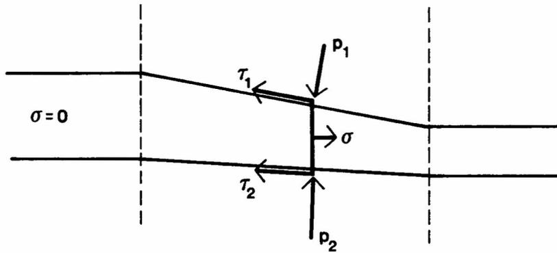
Figure 3. The stresses on the tube.
