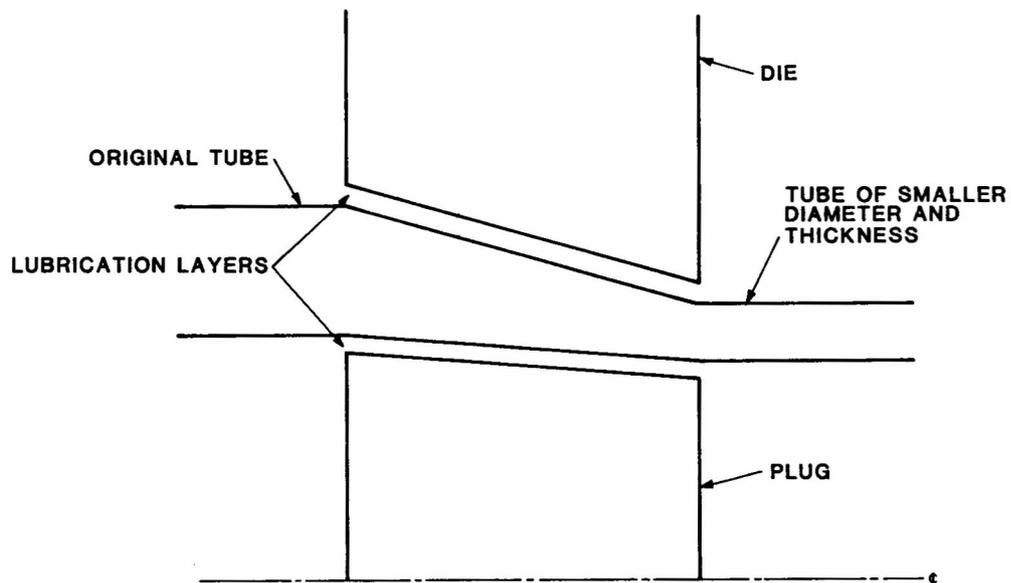
Figure 1. Illustrating the geometry of tube drawing equipment.
