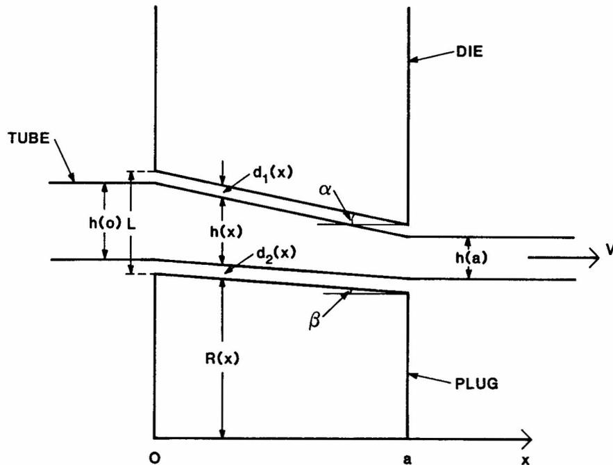
Figure 2. Tube drawing geometry and the definition of variables.
