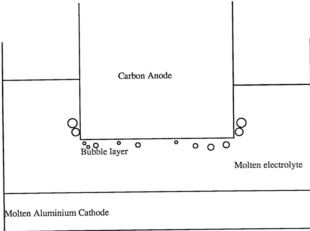
Figure 1: Diagram of one anode block within pot.
