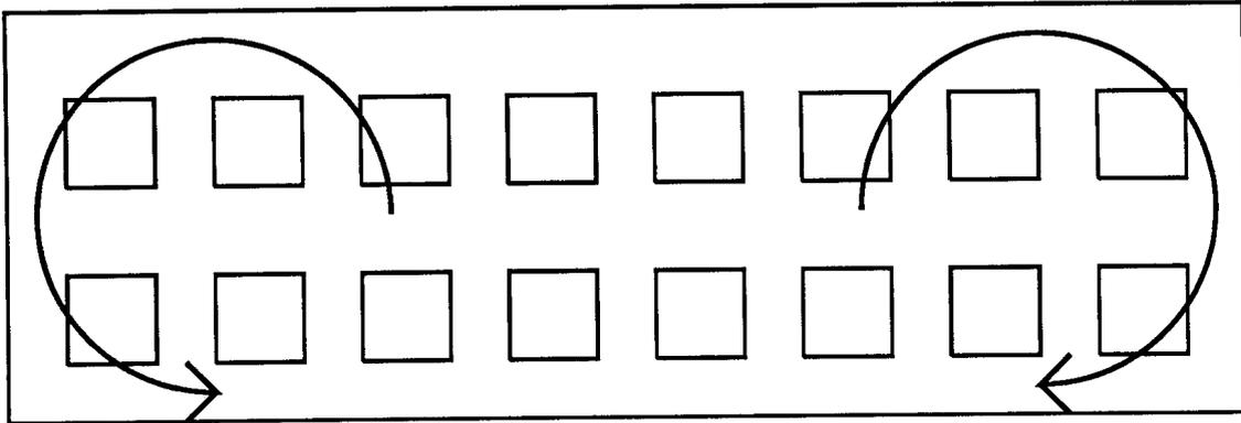
Figure 2: Typical large scale magnetically induced circulation pattern in the electrolyte.
