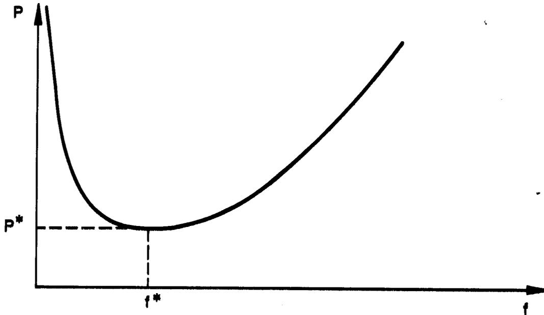
Figure 3: Centre buckling when  $T > 0$
