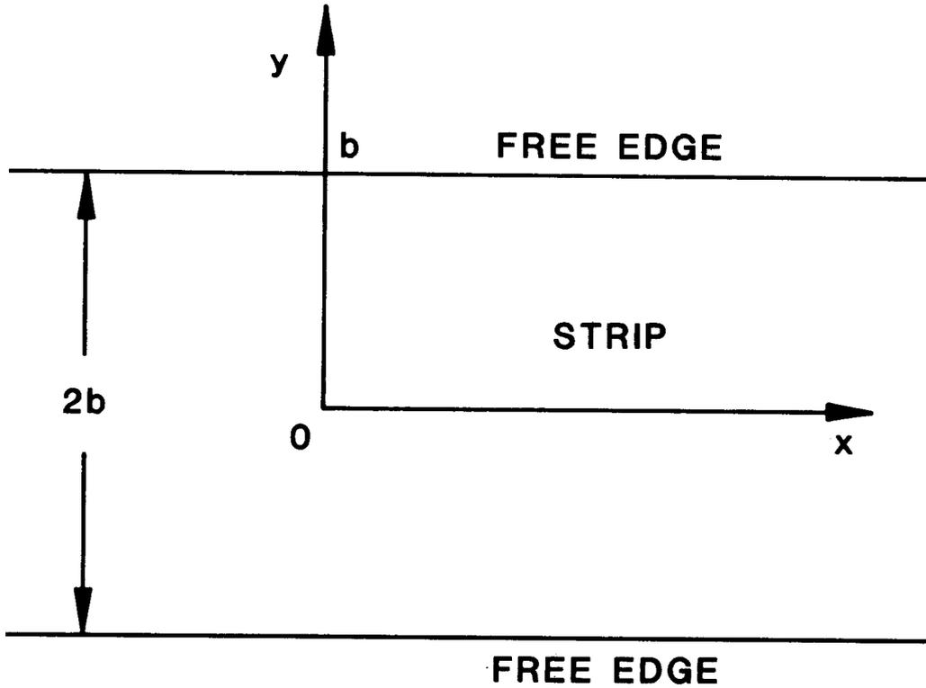
Figure 1: Geometry of strip.
