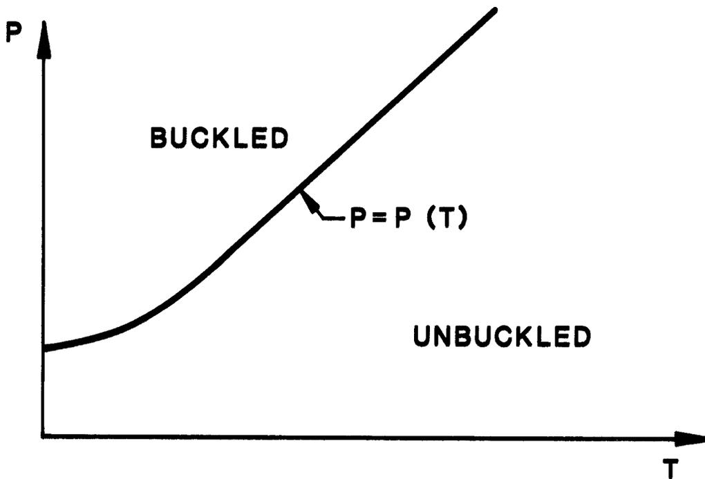
Figure 4:  $P(T)$  versus  $T$  for centre buckling.
