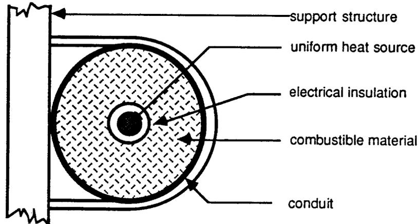
Figure 1: Representation of a cable inside a conduit filled with combustible insulating material.
