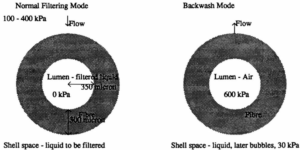
Figure 2: A fibre in cross-section in the two main modes of operation
