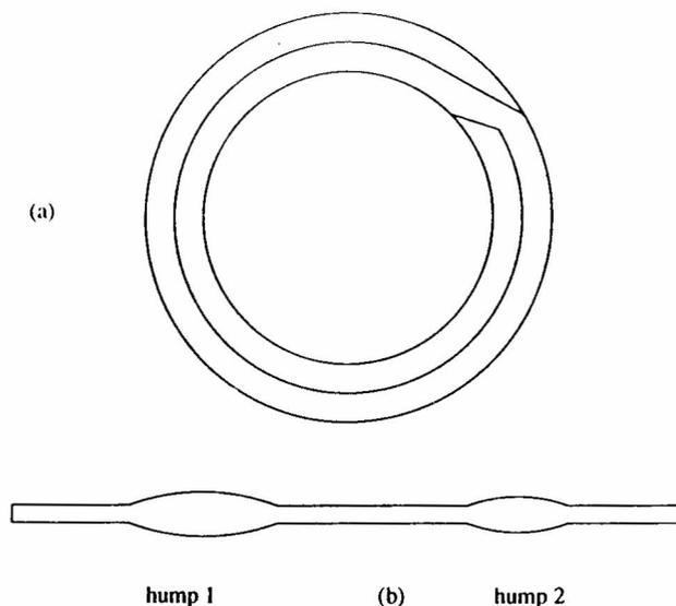
Figure 1: (a) A double wrapped tube. (b) A swimmer. (Different scales.)
