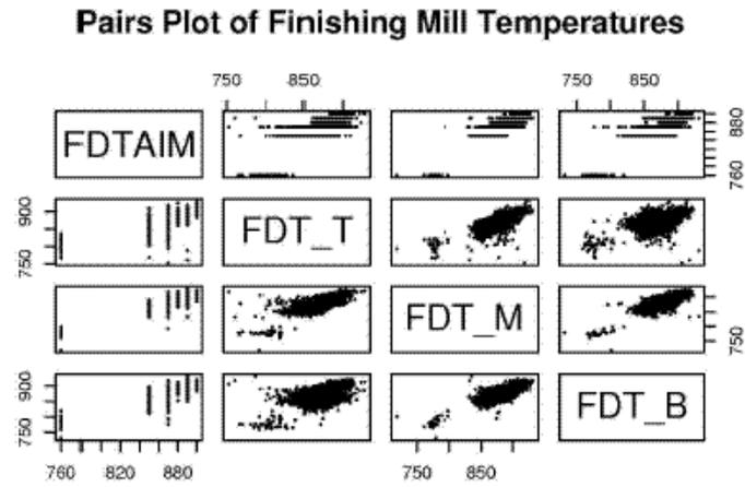
Figure 5. Finisher delivery temperatures
