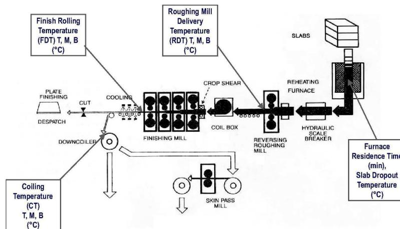
Figure 3. The hot-rolling process.
