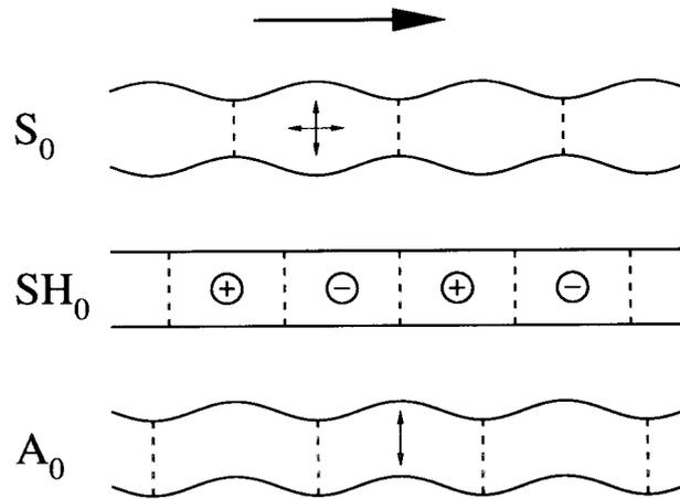
Figure 1: Schematic diagram of plate deformation caused by *symmetrical longitudinal* ( $S$ ) waves, *horizontal shear* ( $SH$ ) waves, and *asymmetrical longitudinal* ( $A$ ) waves.
