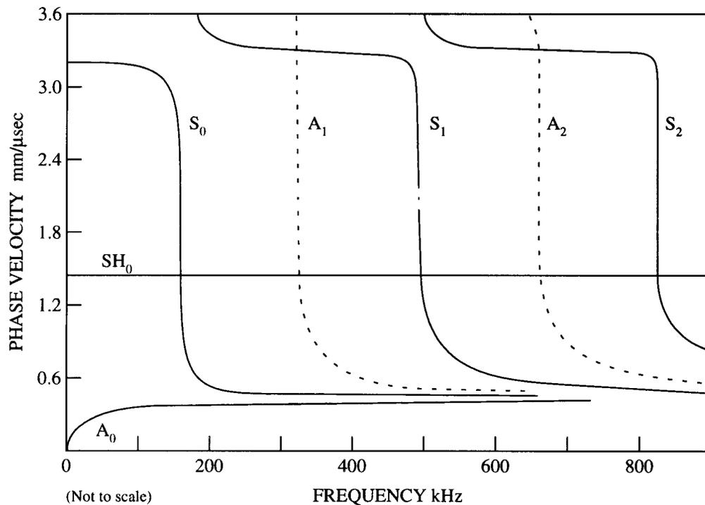
Figure 2: Phase velocity versus frequency curves for waves in the machine direction for an orthotropic plate. After figure 3 of Mann, Baum, and Habeger (1979).
