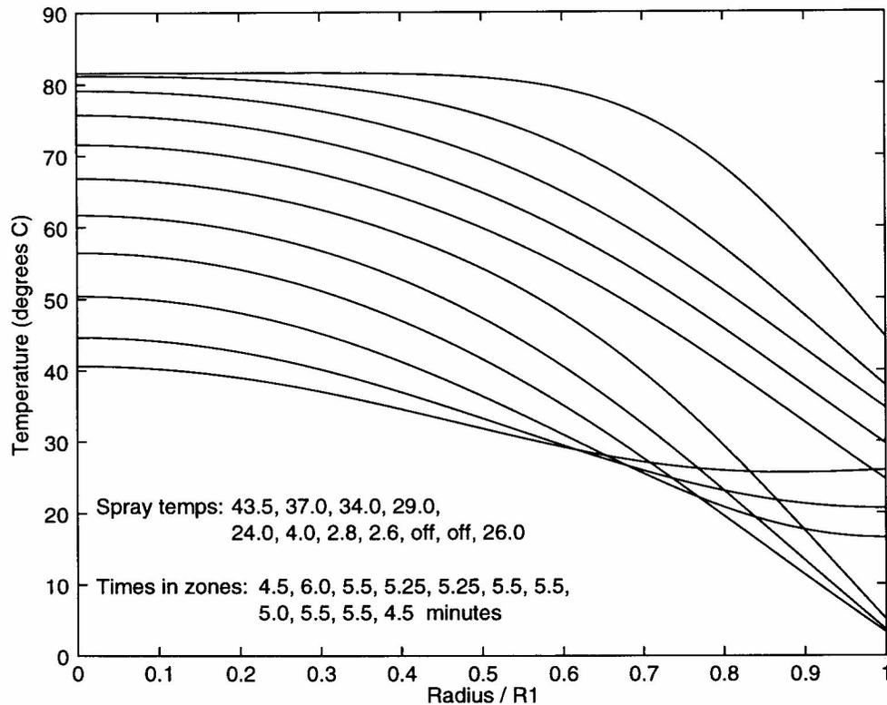
Figure 4: Temperature distribution in the cheese as a function of radius in the 11 cooler zones. The spray temperatures are taken from experiments by Kraft.
