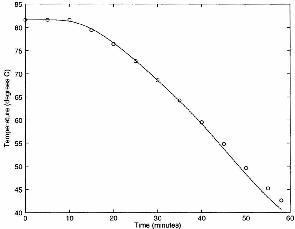
Figure 3: The predicted core temperature of the cheese spread in the jar as it moves through the cooler using the water cooler zone temperatures supplied by Kraft. The circles are the experimentally determined temperatures found by Kraft.
