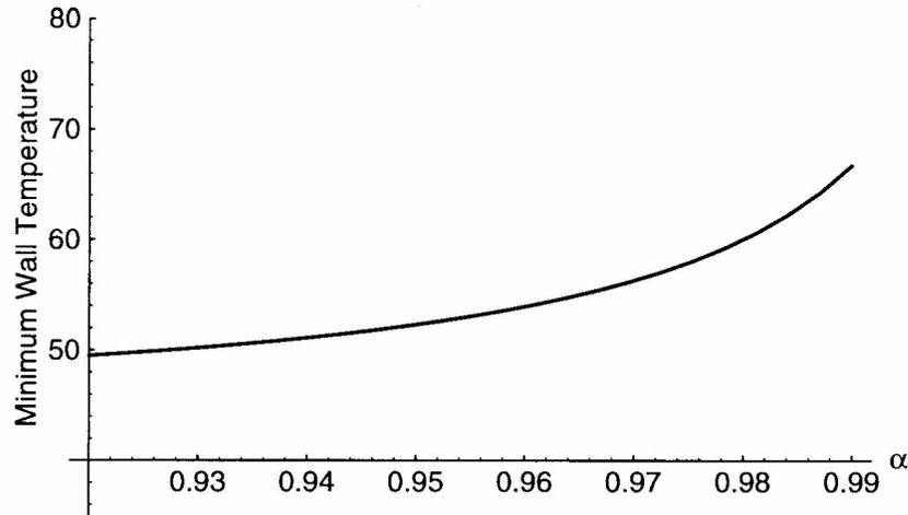
Figure 5: Estimated water temperature at which boiling will occur as a function of the proportion of the jar filled.
