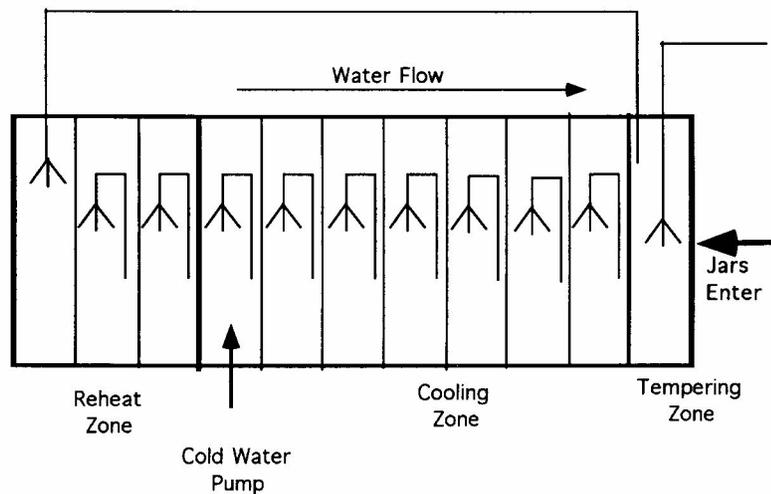
Figure 1: The Kraft 11-zone jar cooler.
