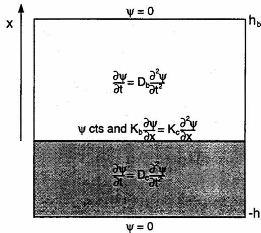
Figure 2: Moisture redistribution equations; subscripts 'b' for belt and 'c' for paste.
