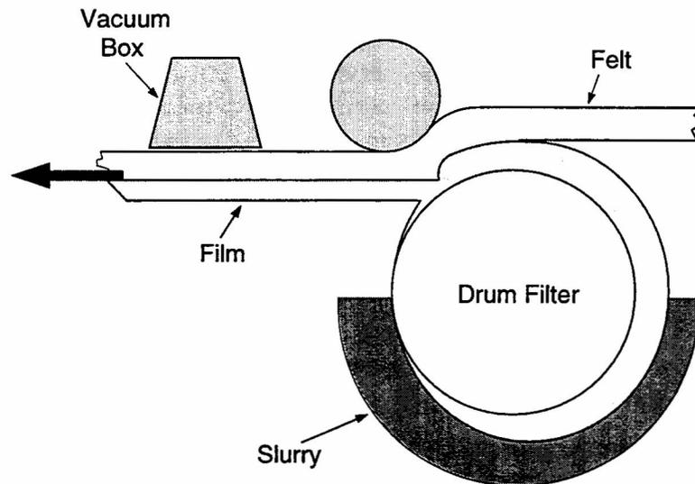
Figure 1: Fibre cement board production.
