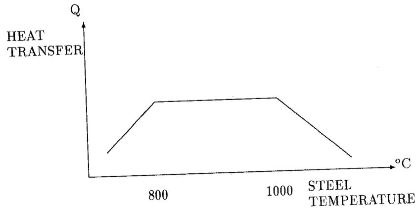
Figure 1: Heat transfer  $Q$  vs. steel temperature for steel cooling at a constant spray rate
