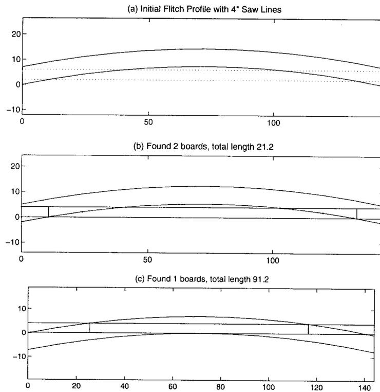
Figure 10: Steps in maximizing length for given width.
