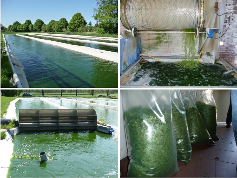
Figure 4.2: Images of an algae farm owned by Ingrepro: Top left, overview of the race-track pond; top right, close up of the mixing device; bottom left, algae extraction apparatus; bottom right, bagged dry algae. Images reproduced with permission of Ingrepro, Borculo, The Netherlands. Website [www.ingrepro.nl](http://www.ingrepro.nl). Photos taken by V.R. Ambati.
