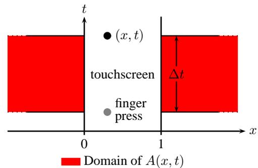
FIG. 8. Domain of integration of equation 21. By causality  $A$  can be non-zero only at times between the finger press at  $(x, t - \Delta t)$  and the response at  $(x, t)$ . Furthermore,  $A$  must be zero for  $0 < x < 1$  i.e. on the touchscreen.
