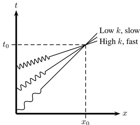
FIG. 6. Ray theory approach to constructing a localised vibration. The medium is dispersive so rays released from a single transducer can be focused on a point.
