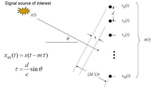
FIG. 10. Array steering.
