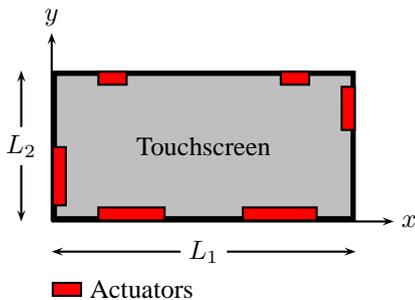
FIG. 1. Geometry of the touchscreen and the transducers. The transducers must be placed at the edge of the touchscreen but can be placed anywhere along the boundary and can be any size.
