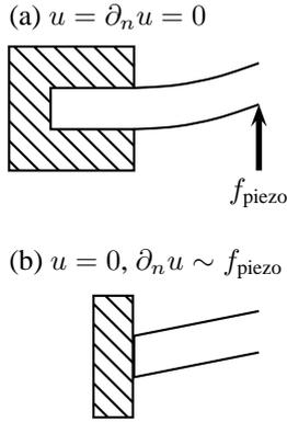
FIG. 5. Choice of boundary conditions. (a) True boundary conditions. (b) Approximate boundary conditions used in this work.
