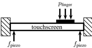
FIG. 3. Schematic of the thin plate model used.
