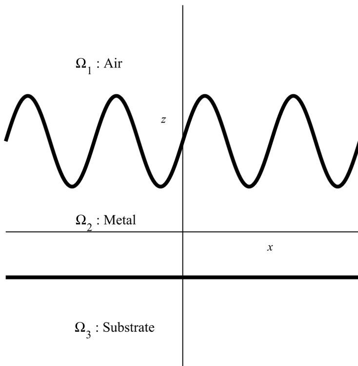
Figure 1: Geometry of the Problem. The  $x$  and  $z$  axes are shown. Since incident electromagnetic waves are supplied in region  $\Omega_1$ , it is convenient to assume that  $z$  increases downward. The  $y$  axis (not shown) should point out of the page by the right hand rule.
