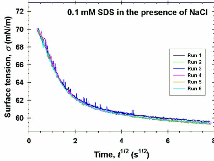
Figure 1: Experimental data for the interfacial tension
