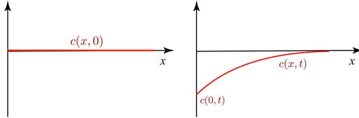
Figure 2: The evolution of the bulk concentration minus its initial value,  $c_{eq}$ . The surface adsorption,  $\Gamma(t)$  grows in proportion to the diffusion flux from the bulk:  $d\Gamma(t)/dt = D \partial_x c(x = 0, t)$
