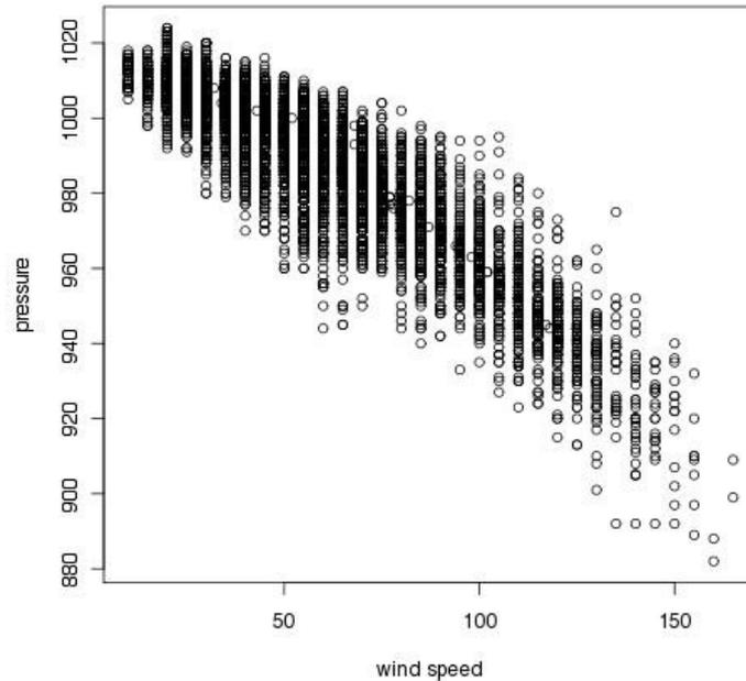
**Figure 1:** Pressure (mBar) vs wind speed (knots) for all hurricanes in the HURDAT data set (1851-2009). Note the strong correlation, but further note that the deepest recession ever recorded did not give rise to the highest wind speed ever recorded.
