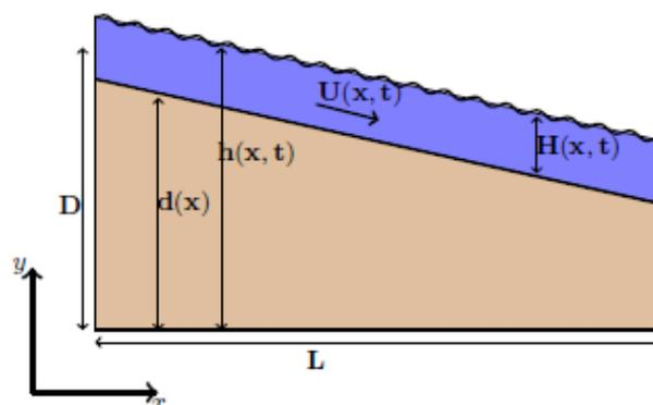
Figure 1: Diagram of modelling set-up including relevant parameters for the shallow water equations
