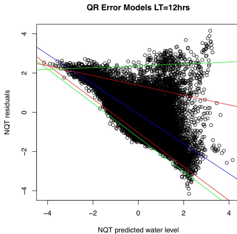
**Figure 3:** Quantile regression with a linear fit. Showing 1st, 5th, 50th, 95th and 99th percentiles.
