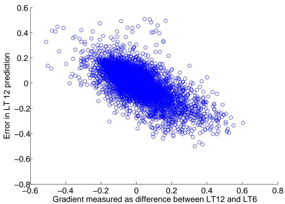
**Figure 2:** Scatter plot of error against gradient as measured by the difference in the LT12 and LT6 predictions.
