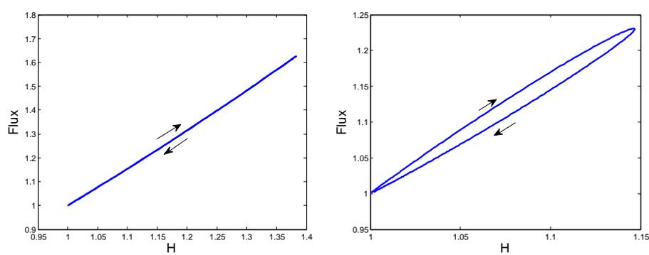
Figure 3: Plots of water flux against depth of the river at a fixed location as a flood passes through (arrows show increasing time).  $\epsilon = 0$  is on the left, with  $\epsilon = 0.02$  on the right.
