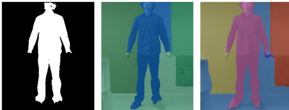
**Figure 7:** Left, current segmentation. Centre, SWA only. Right, SWA with Perona-Malik. SWA achieves a similar quality to the current Poikos segmentation
