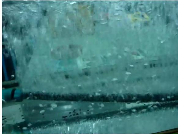
Figure 4: The bubble flow from the aeration tube
