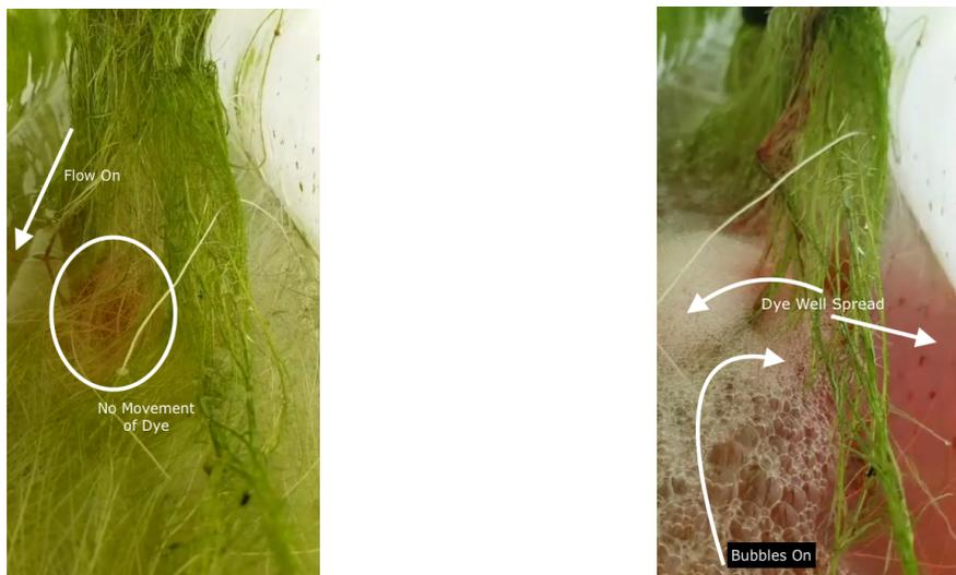
(a) Main inlet flow turned on. No movement of dye observed. (b) Bubble flow turned on. Good spread of dye observed.
