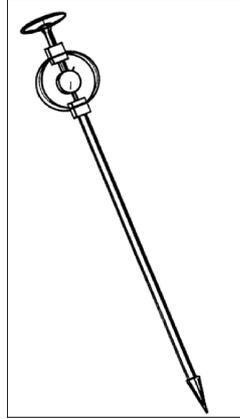
Figure 18. A modern penetrometer [3]
