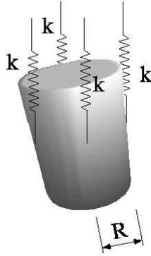
Figure 3. Pictorial representation of the radius of the bowl and stiffness of the springs
