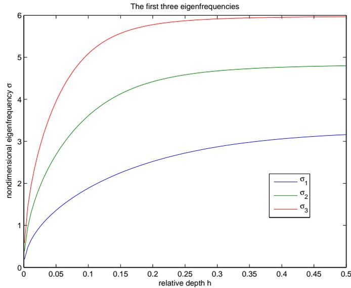
Figure 6. The first 3 eigenfrequencies as a function of relative radial depth  $h$ . We used  $L/R = 2\pi/24$  which corresponds to an average relative cell length when there are 24 cells.
