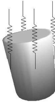
Figure 2. Sketch of the bowl being supported by springs
