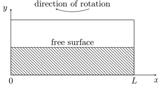
Figure 5. Simplified cell geometry and local co-ordinate system
